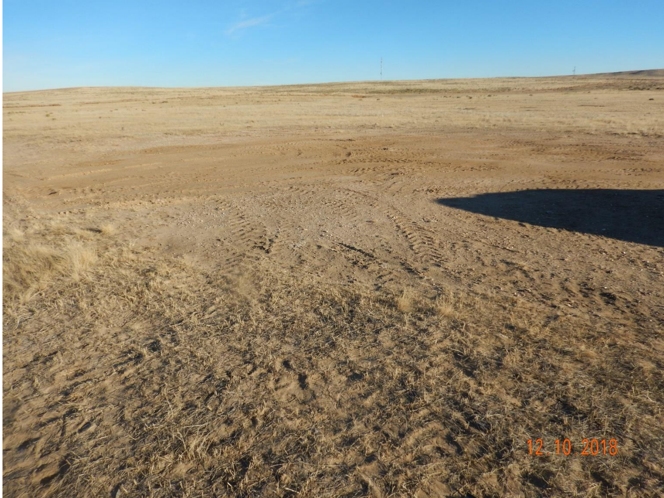
Photo 12: Photo taken from the west end of the battery location, facing northeast. Photo shows operator appears to have spread soil on top of the location, however, gravel has not been removed, compaction alleviation has not been conducted. Reclamation activities do not appear to have been conducted in accordance with 1004 rules and corrective actions.
