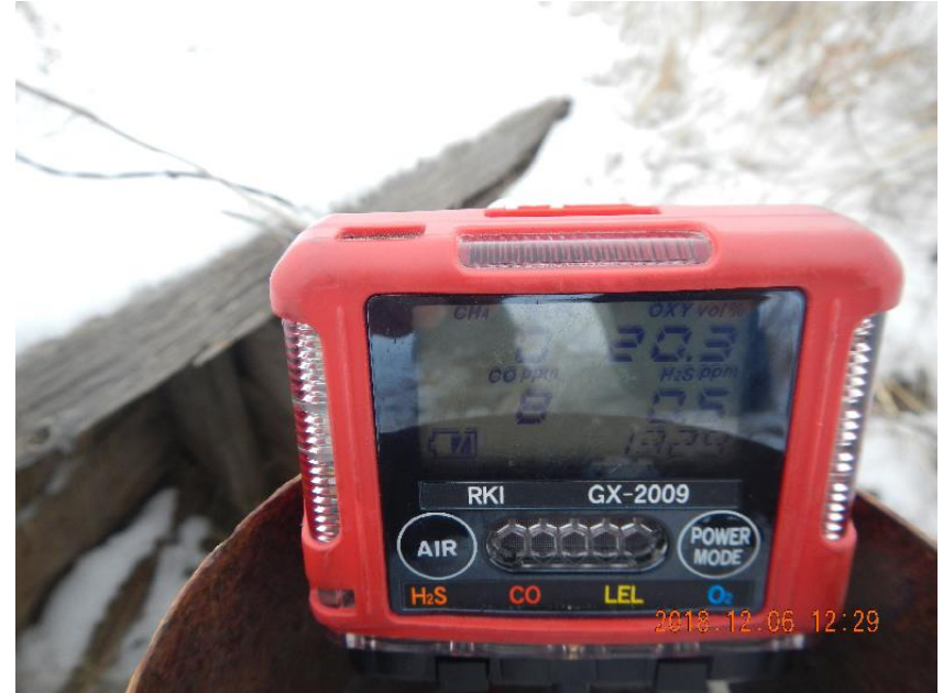
Photo 10: 4 Gas Meter reading at open end of casing. Casing froze off at surface.
