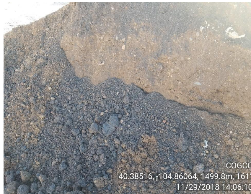
Photo 2 – Hydrocarbon impacted soil along edge of excavation.
