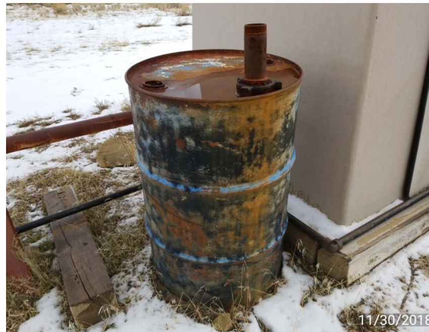
Photo 8. Barrel of fluid stored on location without label or secondary containment.
