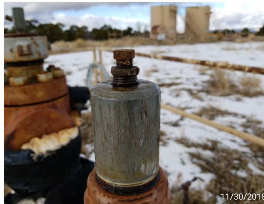
Photo 6. Wellhead bull plug leaking gas along threads of small plug on top of bull plug.
