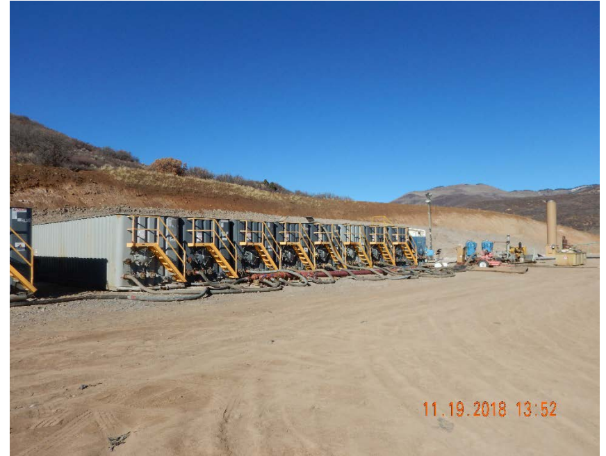
Photo #2 – Frac tanks located along southwest side of pad. Note: frac tanks lacked stormwater control BMPs on inspection date.
