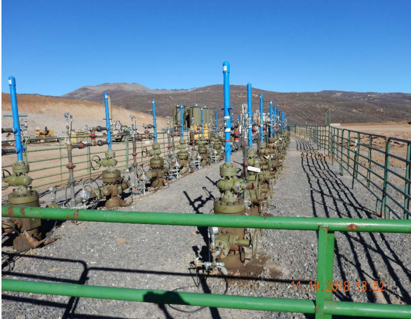
Photo #7 – View of wellheads from south side. Note accumulations of oil-stained soil at base of wellheads.
