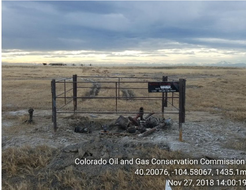
Photo 1 WH unused equipment around P&A well
