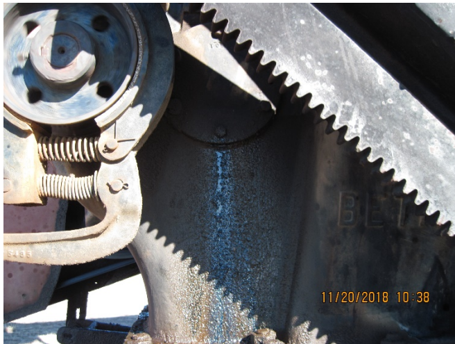
3. Origin of oil, gear box cover gasket leak
