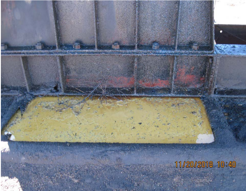
5. North side of unit base, bull shaft gasket leak
