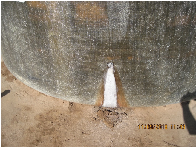
3. Tank leaking
