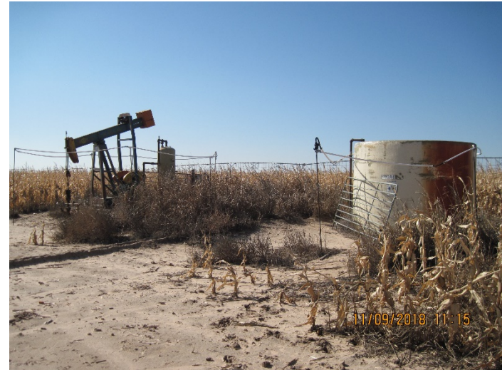
4. Pumping unit, Tank with inadequate berms, weeds
