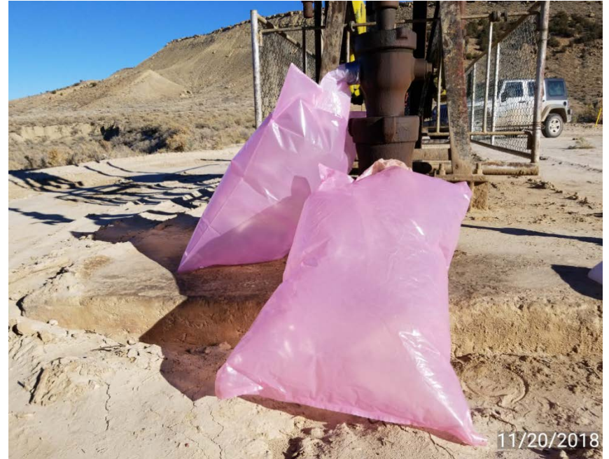
Photo 3. Gas collection bags attached to both vent openings.
