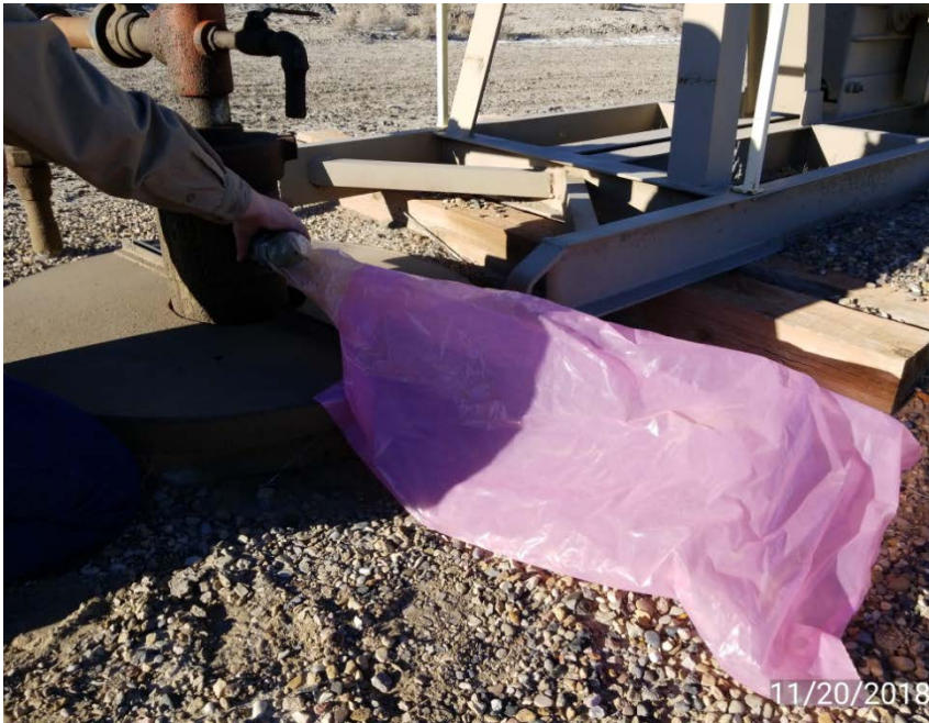
Photo 3. Gas capture bag attached to well head.
