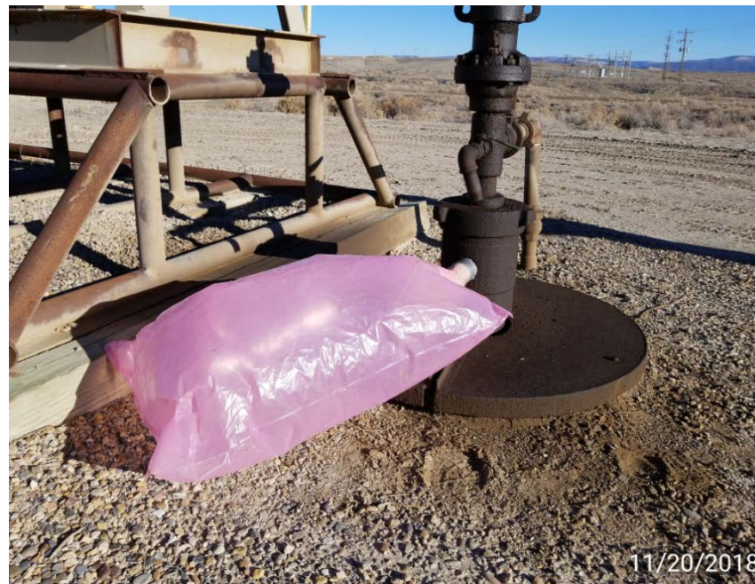
Photo 2. Gas capture bag attached to well head.
