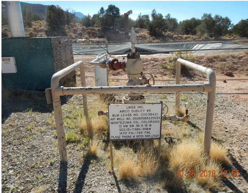
Airco Dudley #5 well head and location sign. Location sign is missing 24 hour contact number and emergency number.
