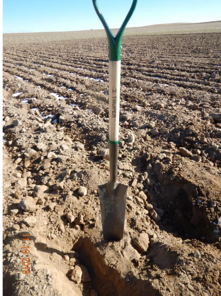
Photo 6: Photo taken from the location. Photo shows inspector tested the location for compaction. Photo shows inspector was only able to penetrate the top couple of inches of soil on the areas of location that were not ripped. Compaction concerns evident.
