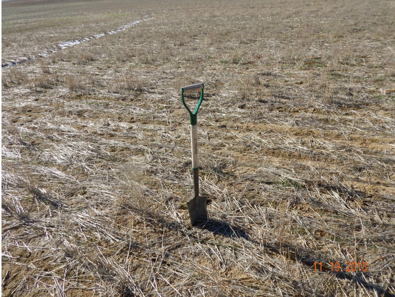
Photo 9: Photo taken from the adjacent reference area. Photo shows inspector was able to easily penetrate the top 6-8 inches of soil.
