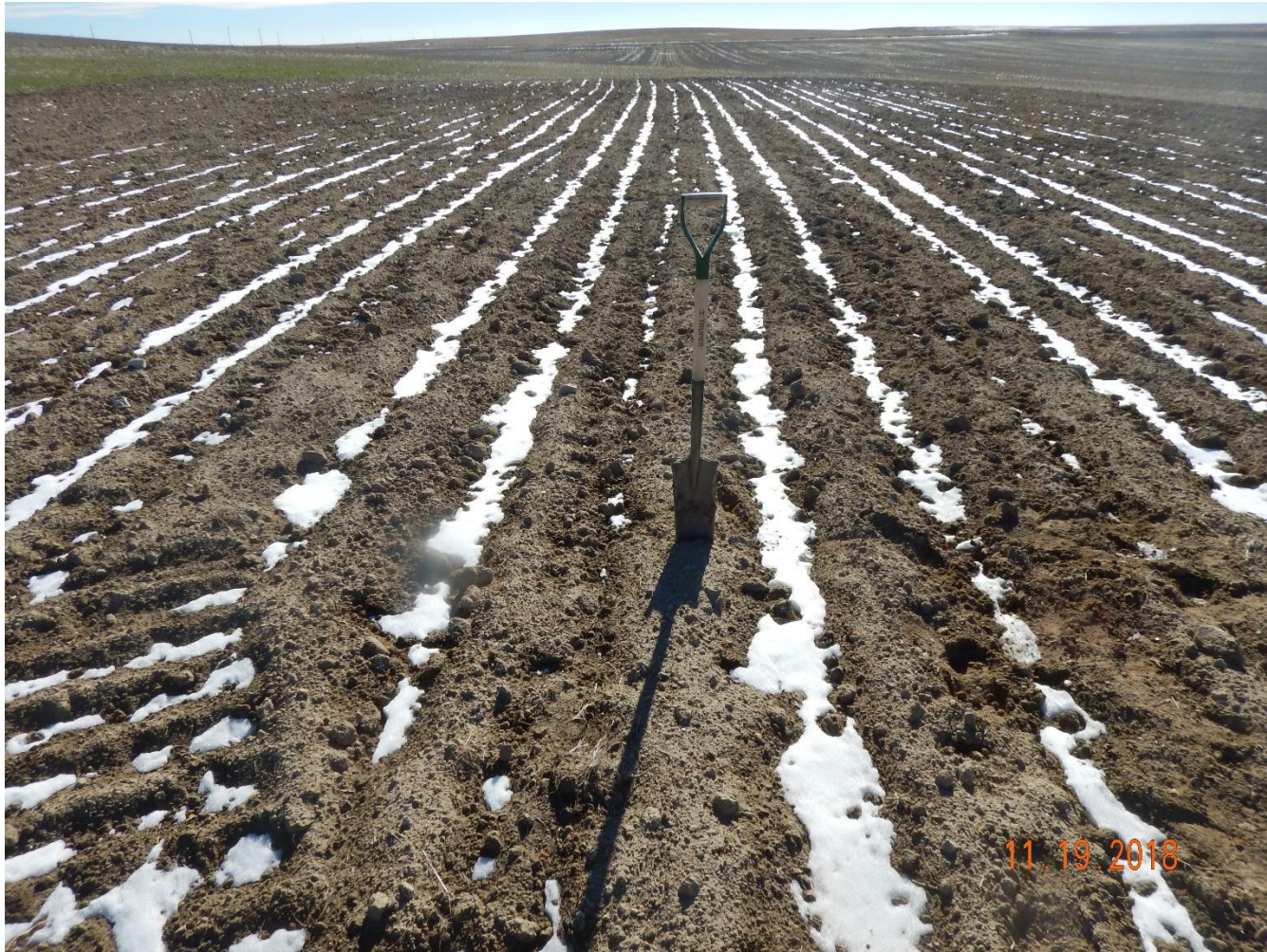
Photo 10: Photo taken from the location, facing south. Photo shows inspector tested the location for compaction. Photo shows inspector was only able to penetrate the top couple of inches of soil on the areas of location that were not ripped. Compaction concerns evident.
