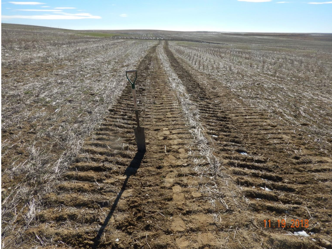
Photo 8: Photo taken from the access road, facing south. Photo shows inspector tested the access road for compaction. Photo shows inspector was only able to penetrate the top inch of soil on the access road. Compaction concerns evident.
