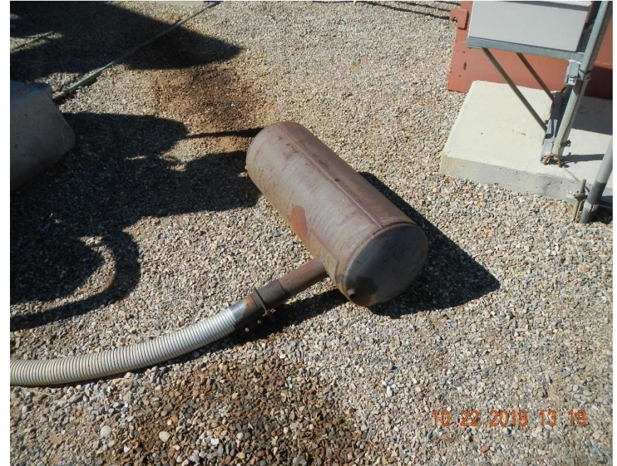
Stained gravel near pump jack exhaust.
