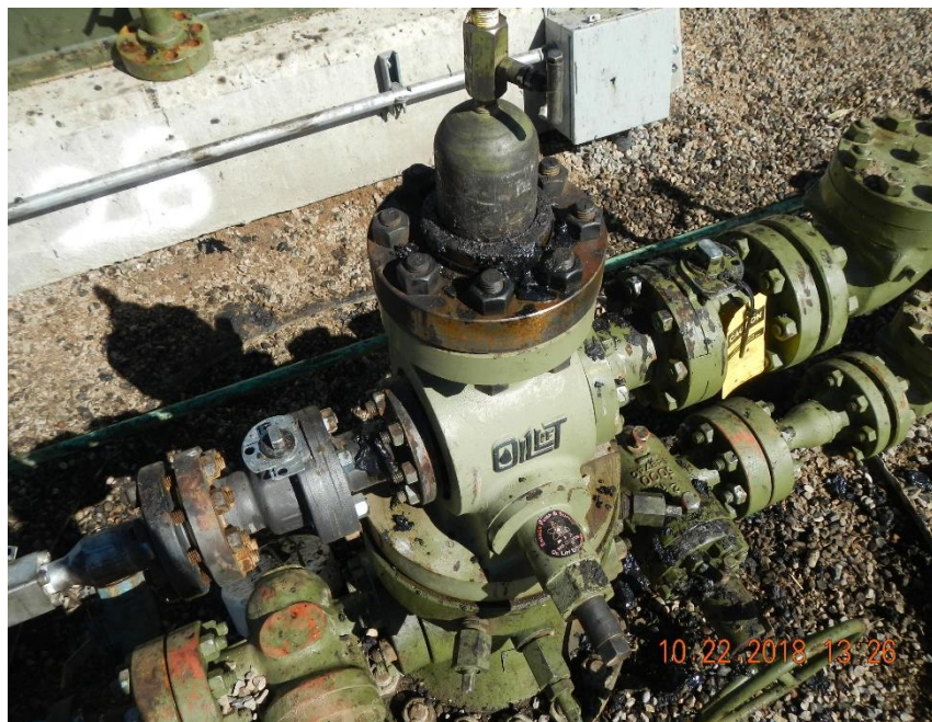
Well head and surrounding gravel are stained and wet.
