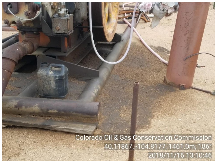
PHOTO 5: STAINED SOIL AROUND PRIME MOVER & INSIDE SKID.
