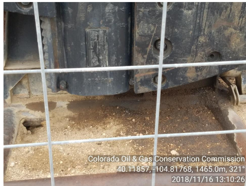
PHOTO 4: STAINED SOIL UNDER GEARBOX ON PUMPING UNIT
