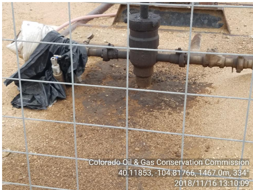
PHOTO 3: STAINED SOIL AROUND WELLHEAD
