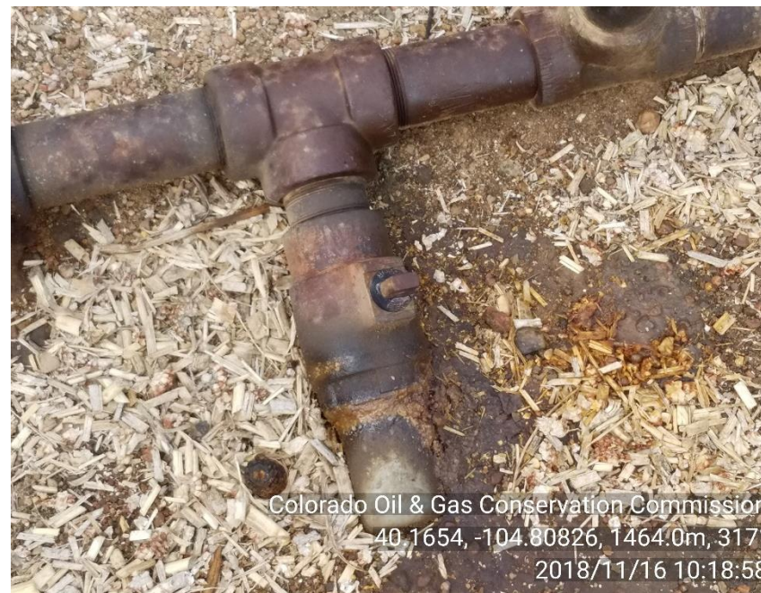
PHOTO 2: VALVE & BULLPLUG LEAKING
