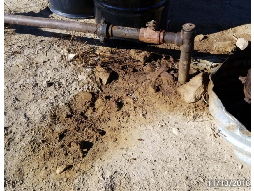
Photo 6. Oily waste on ground near wellhead
