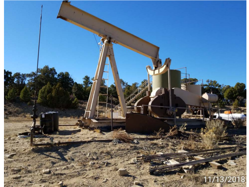
Photo 2. Pump jack is partially disassembled.
