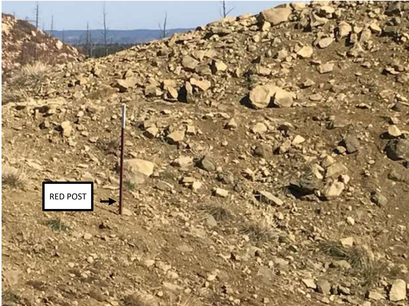
A RED POST WAS INSTALLED IN THE PRODUCTION PIT TO MONITOR (2) FOOT OF FREEBOARD BETWEEN THE TOP OF THE PIT WALL AND THE FLUID LEVEL OF THE PIT.
