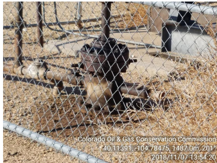
PHOTO 2: wellhead wet with fluid/ stained soil around wellhead
