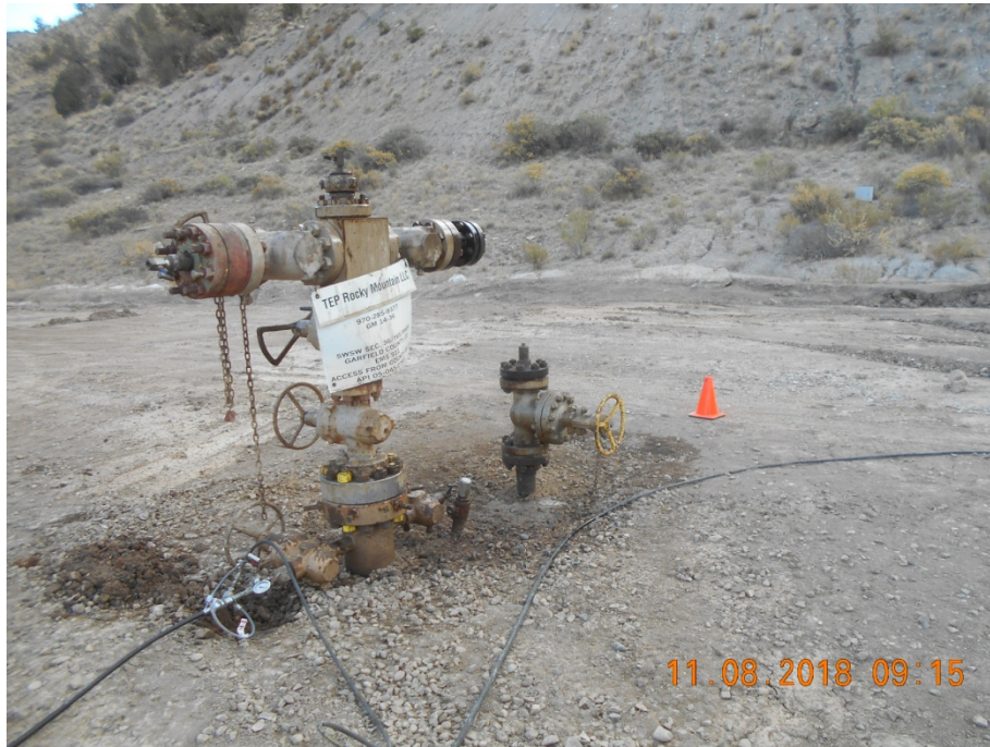
Injection wellhead
