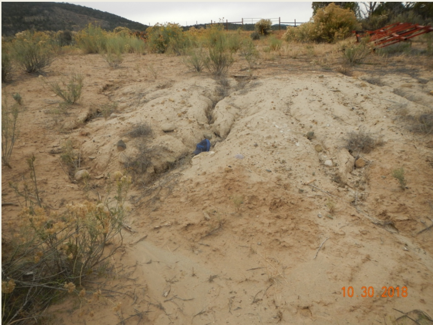
Photo 5. View of erosional channels up to 18 inches wide and deep within the northeastern project area.
