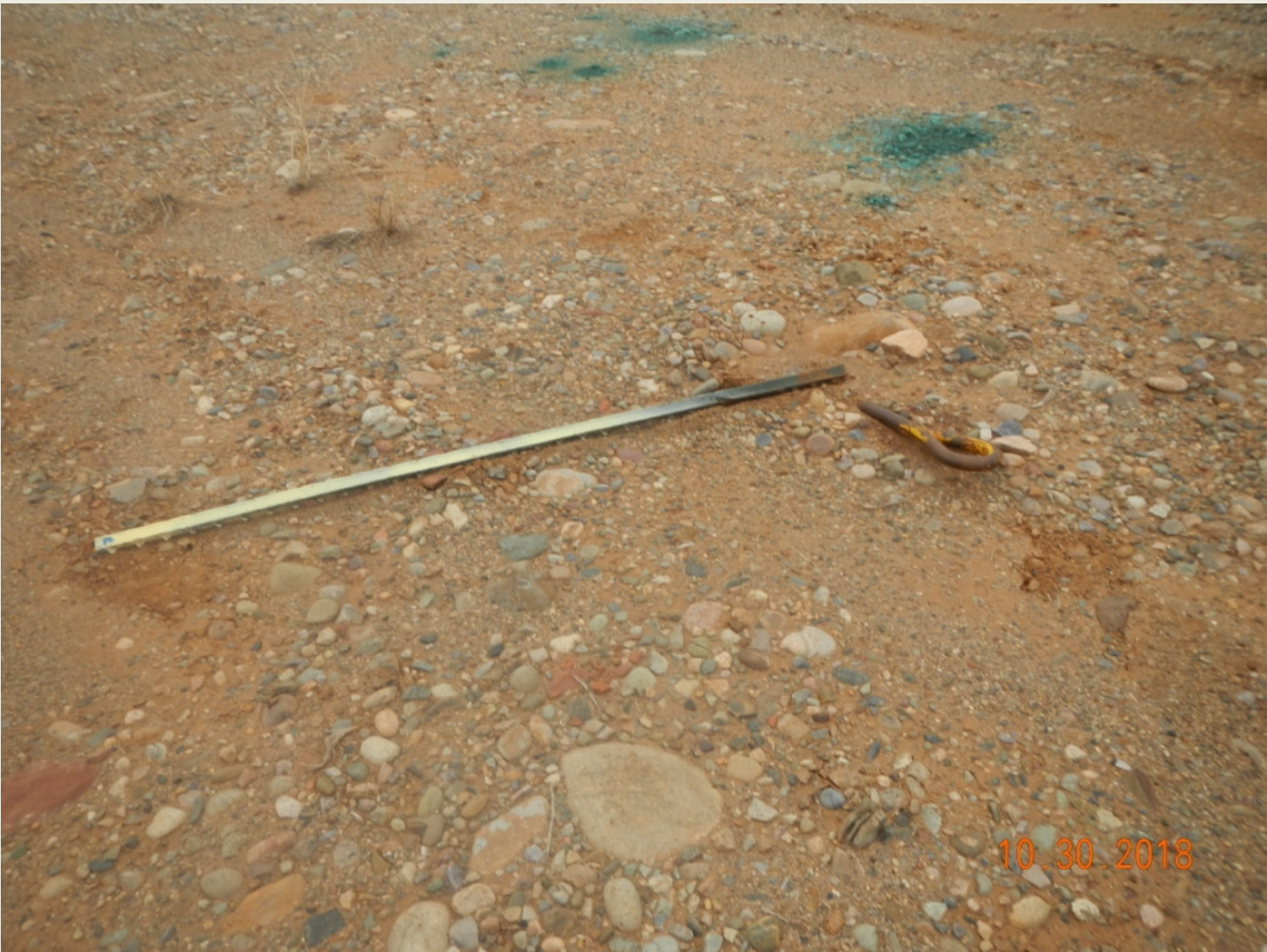
Photo 4. View of rig anchor an marker (broken) within the working area.
