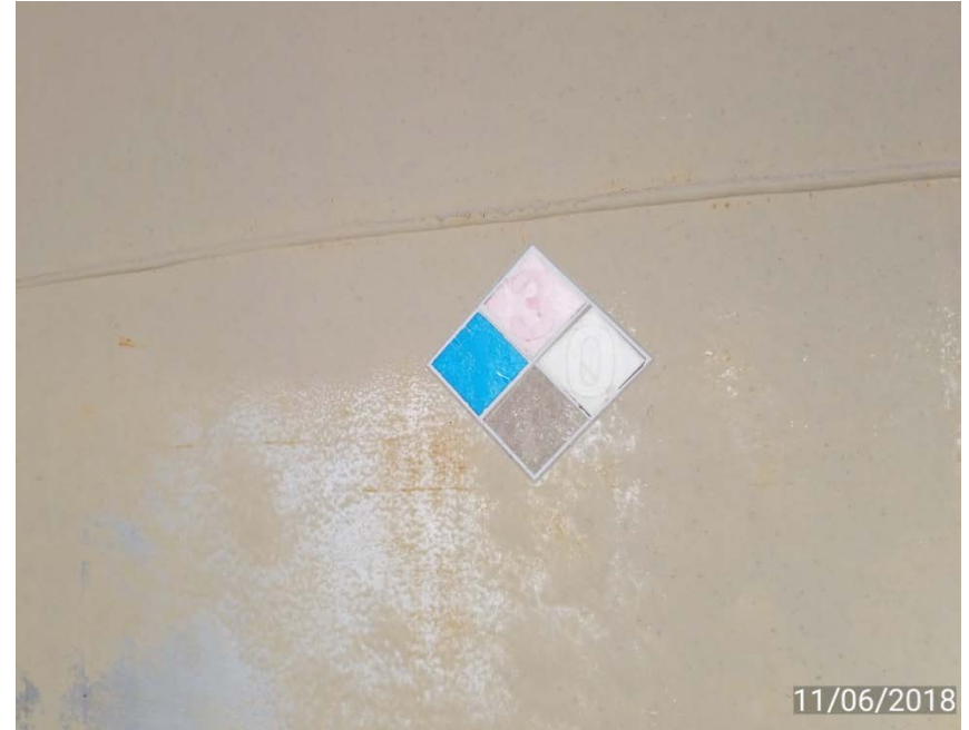
Tank without NFPA label, contents, capacity of 300 bbl, operator, and phone number.
