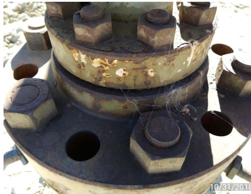
Gas leaking out at well head bolt holes
