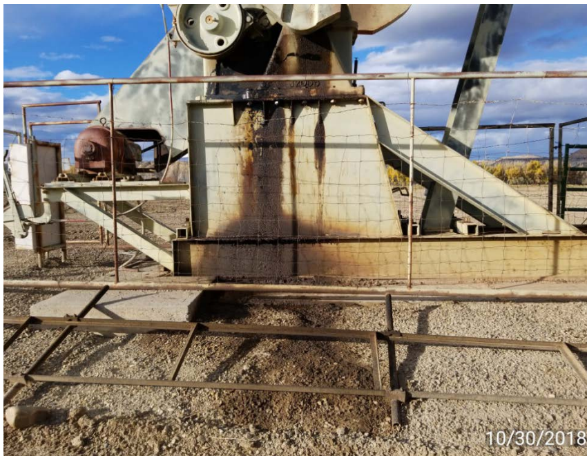
Oil on pump jack - north side
