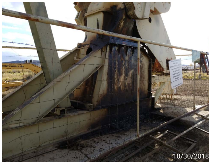
Oil on pump jack - south side
