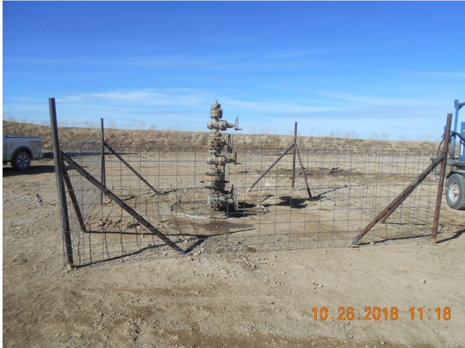
Wellhead with fencing
