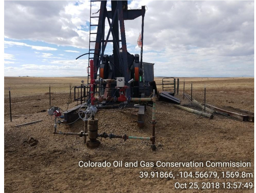
Photo 2 WH PU disconnected plunger lift installed PU unused equipment
