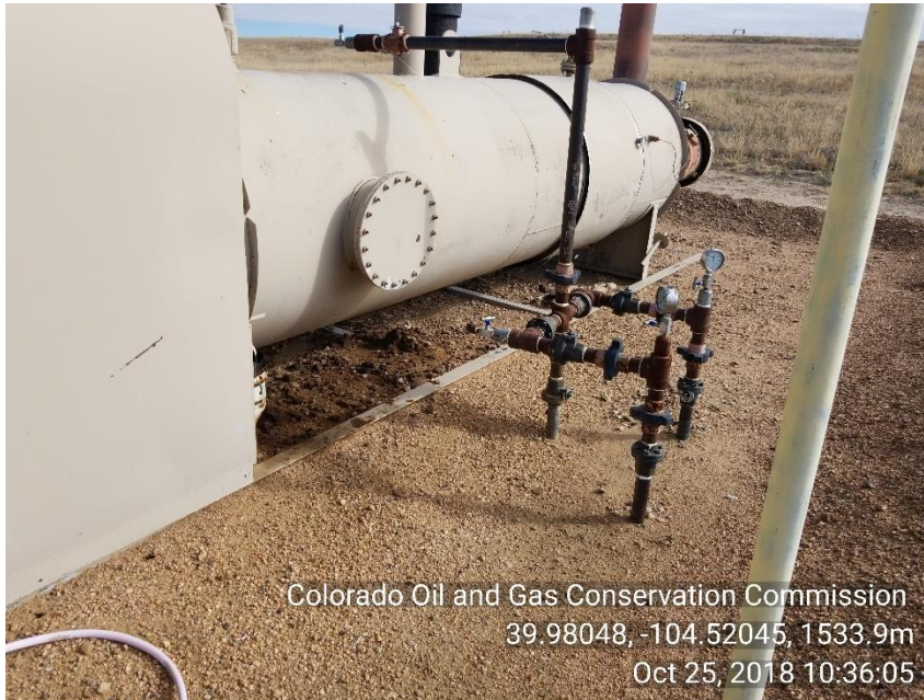
Photo 3 Stained soil under sep drain lines
