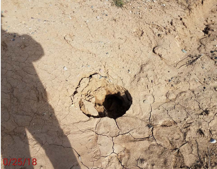
Location Photo #5, Storm water draining into holes along the ditch.
