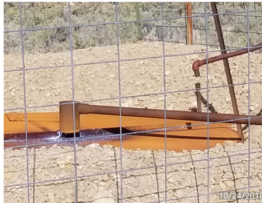
Separator venting to tank during first 5 minutes while inspector on location.
