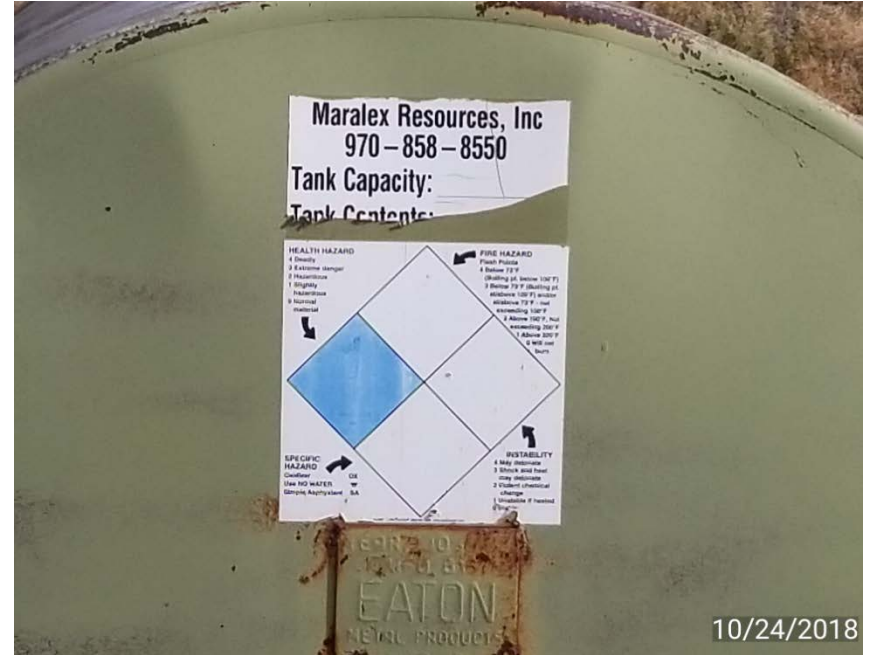
Tank with missing capacity, contents, and NFPA label.
