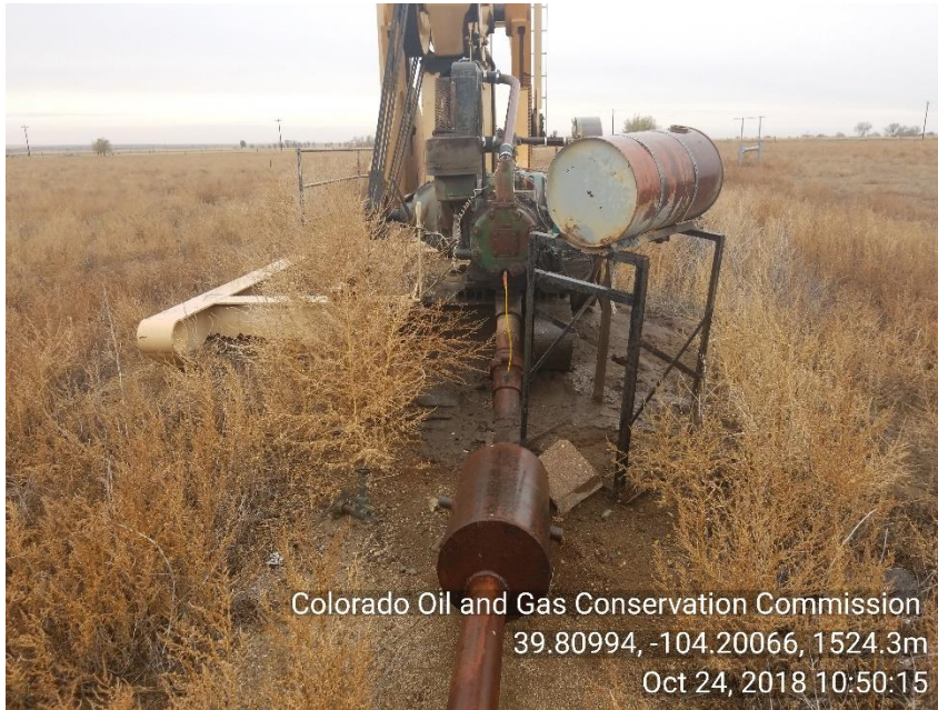
Photo 3 Stained soil PU exhaust
