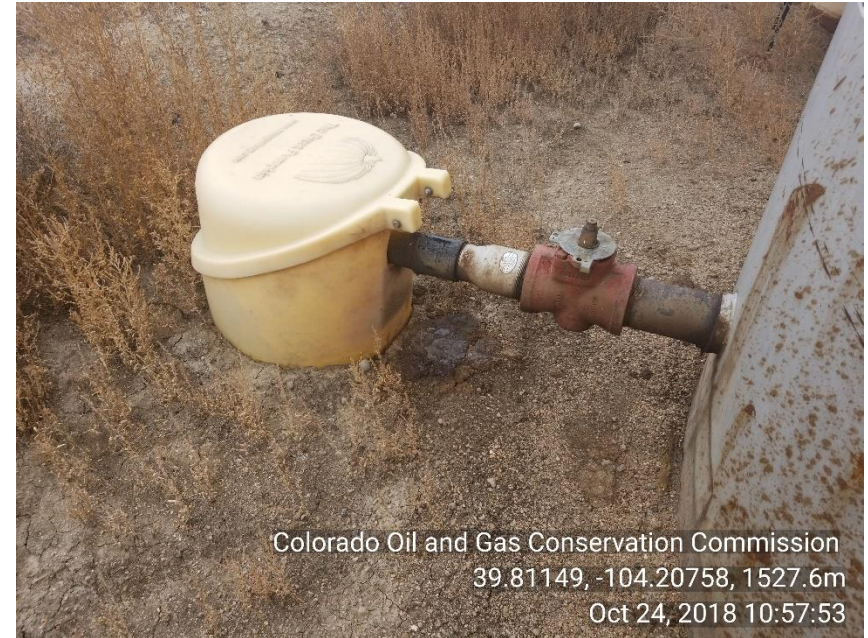
Phot 10 Stained soil under load out line to pro water tank
