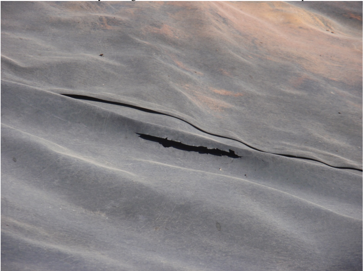
Photo 26. Visible tear in liner on south side of pit.
