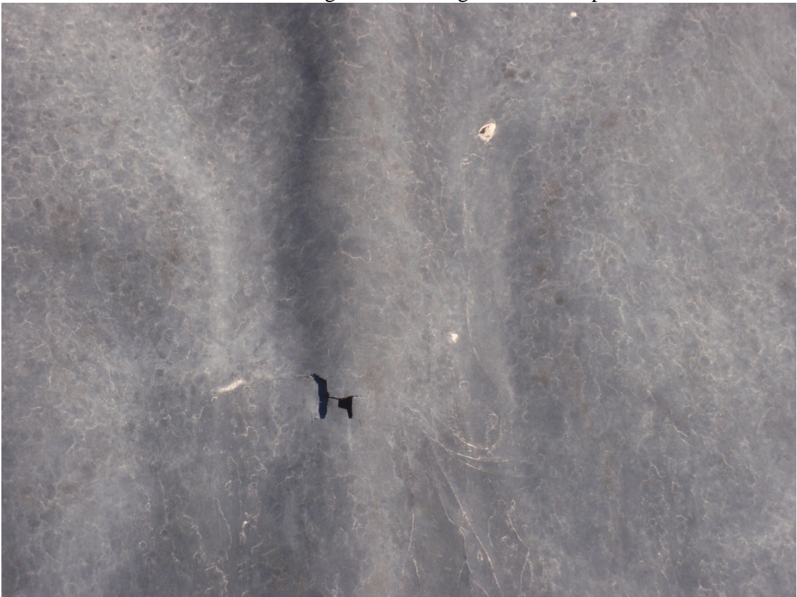
Photo 62. Damage to liner along north side of pit
