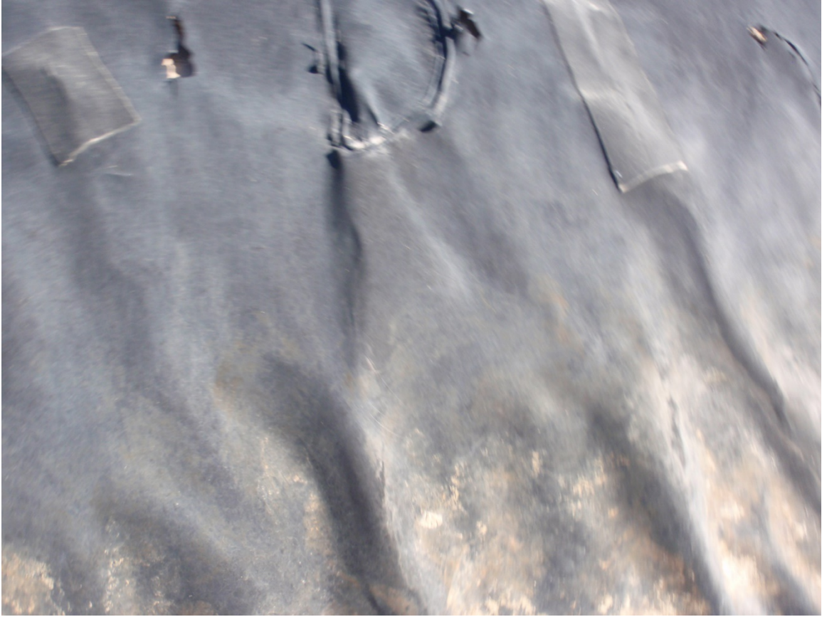
Photo 77. Damage to liner along north side of pit
