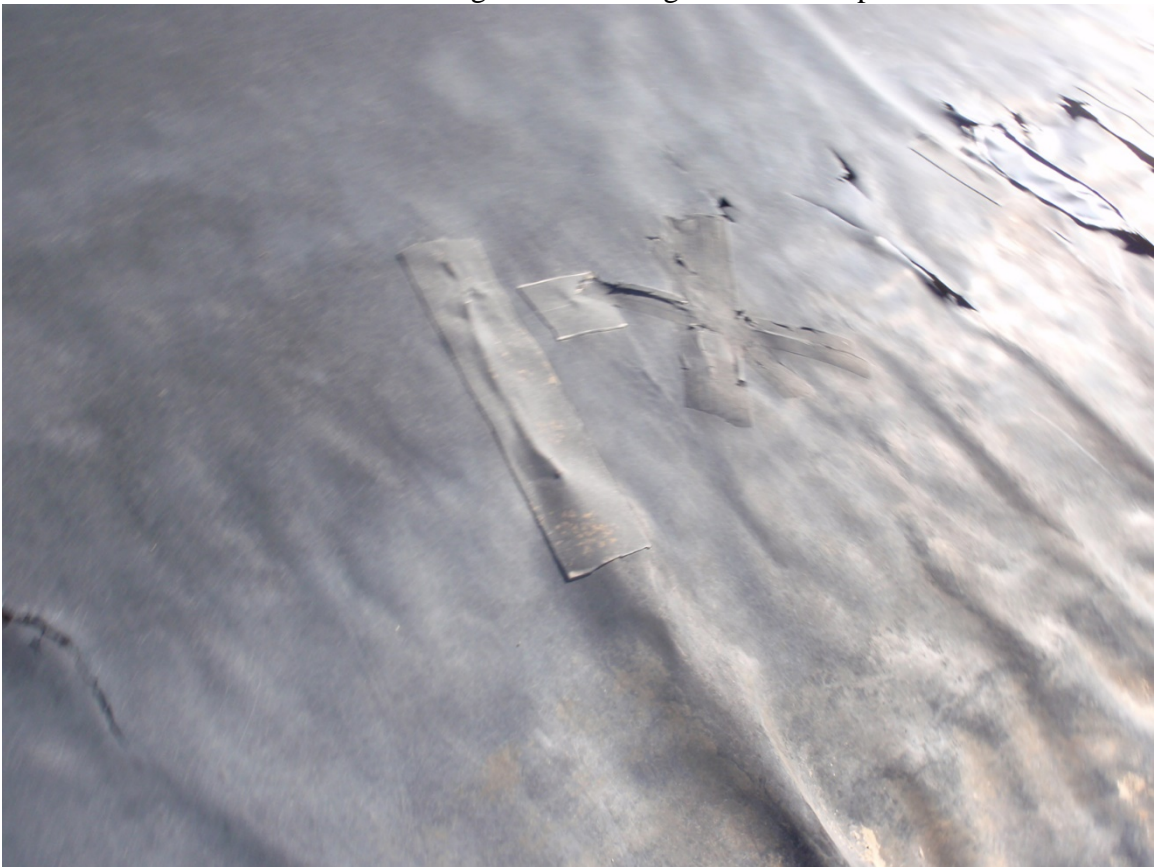
Photo 78. Damage to liner along north side of pit
