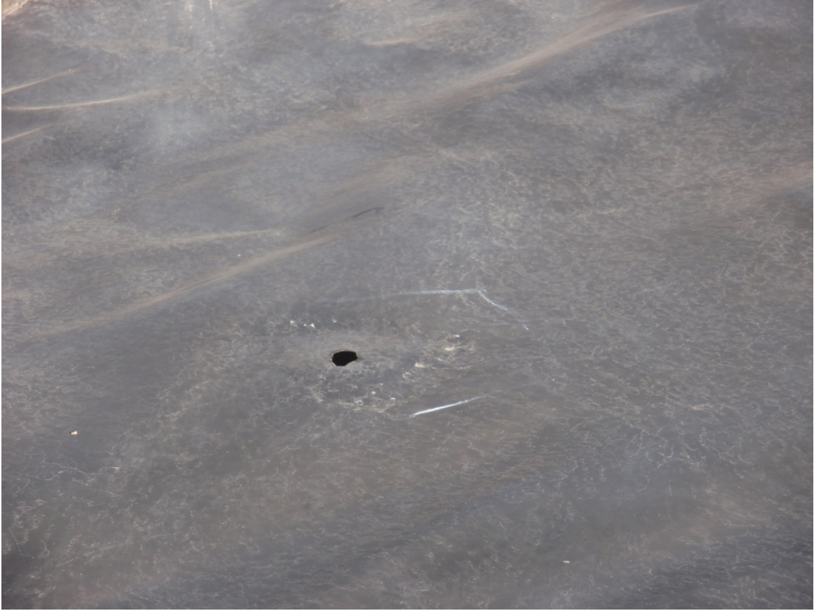
Photo 104. Small hole in liner on east side of pit
