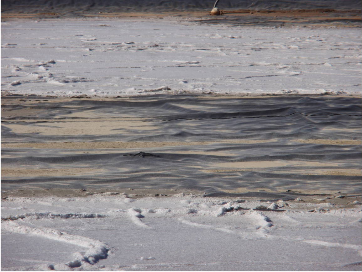
Photo 102. Accumulation of sediment and salt in middle of pit.
