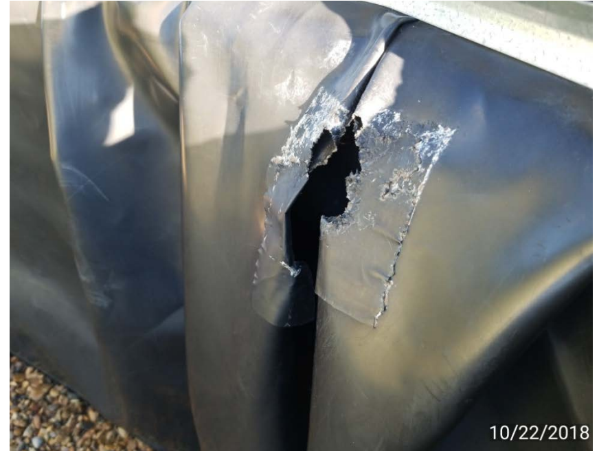
Hole in tank liner
