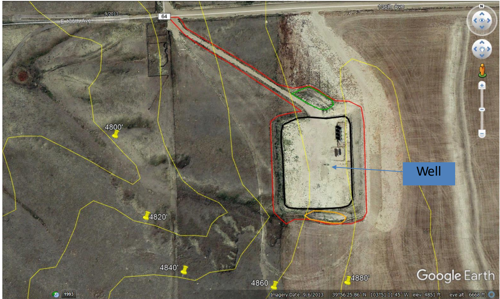
Photo 3: 9/06/2013 aerial imagery. 2A doc. #400252948 states size of location after IR is 0.92 acres, with IR estimated to begin on 9/1/2012. Based on production records, interim reclamation (IR) on areas no longer reasonably needed for production should have occurred no later than 10/2012. Photo image date is 11 months after when IR should have occurred. Photo shows location does not appear to have been reduced in size; IR does not appear to have been conducted. Total disturbance remains ~4.9 acres with pad/production area ~2.43 acres.
