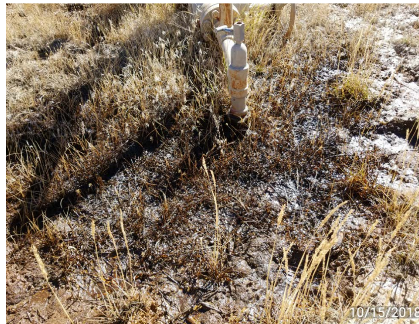
Oil on ground next to well head
