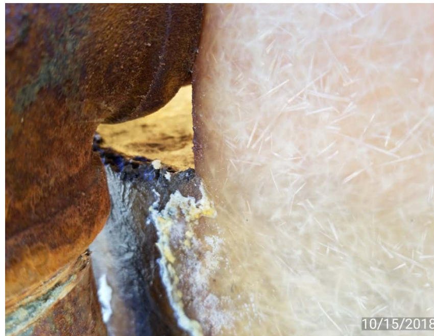
Tank leaking fluid with oil on top of produced water.
