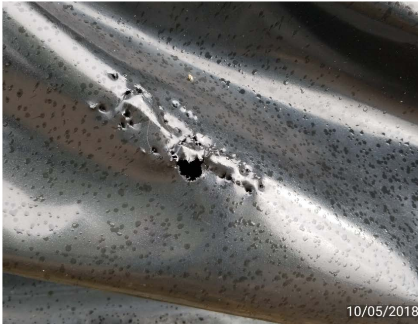
Holes in berm liner
