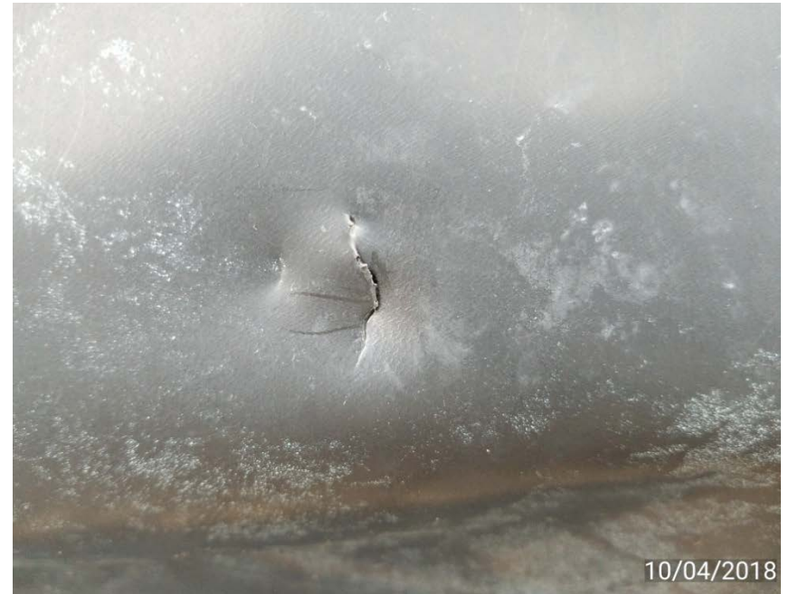
Tear in tank liner
