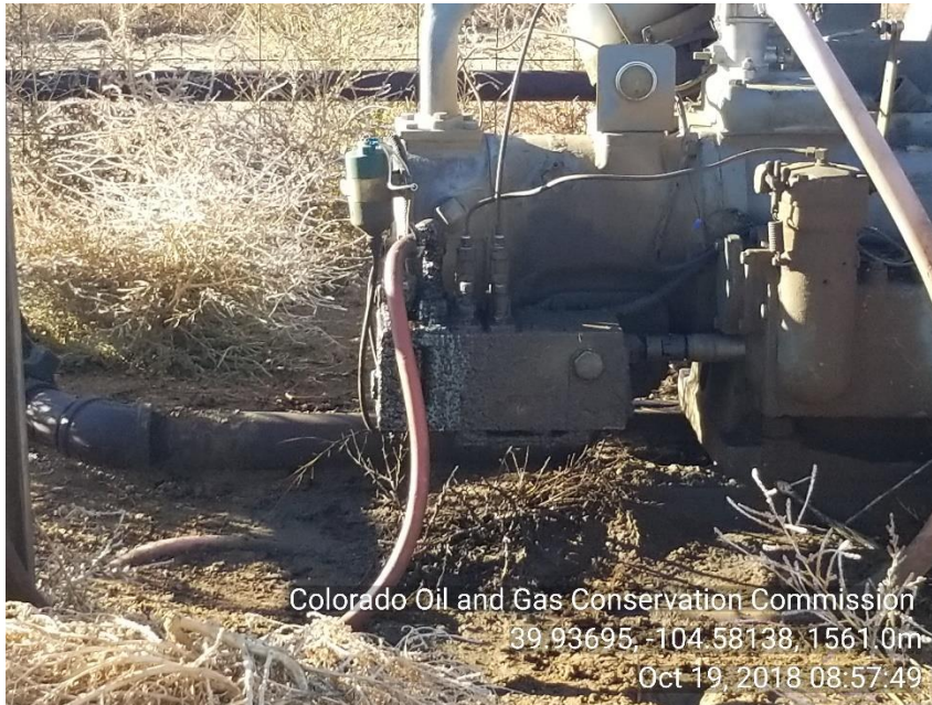
Photo 3 Stained soil under motor of PU
