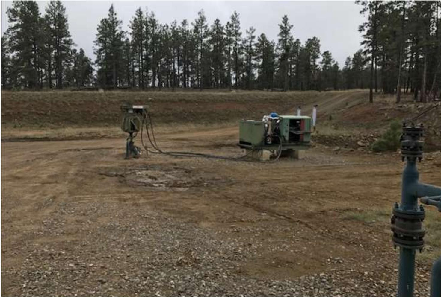
WORKOVER OPERATIONS ARE COMPLETE FOR THIS WELL. ALL RODS AND PIPES HAVE BEEN REMOVED FROM LOCATION. THE PUMP DRIVE WAS REPLACED AND THE WELL IS BACK ON LINE.
