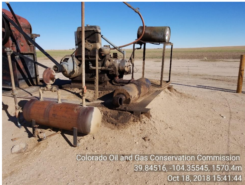
Photo 3 Stained soil exhaust
