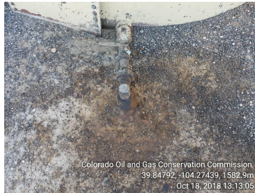
Photo 4 Stained soil crude oil tank
