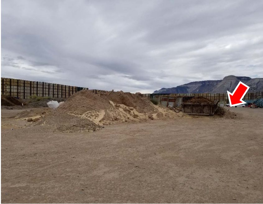
Photo #17 – Overview of NE Special Waste Stockpiles from NE corner of pad. Note lack of stormwater control and presence of stained soil outside of metal container (red arrow).
