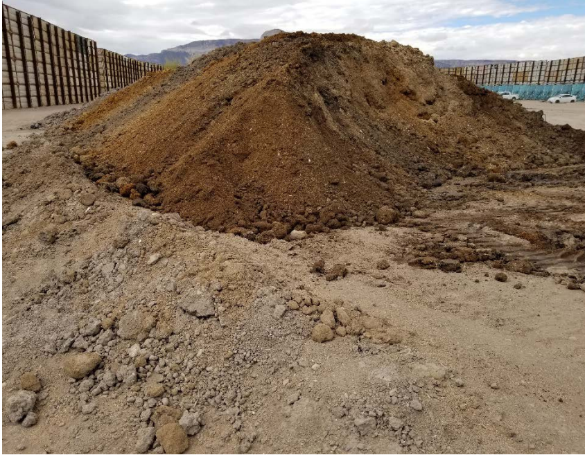
Photo #11 – View of SE Special Waste stockpile from east side. Note absence of earthen berm and presence of equipment tracks on this side of stockpile.
