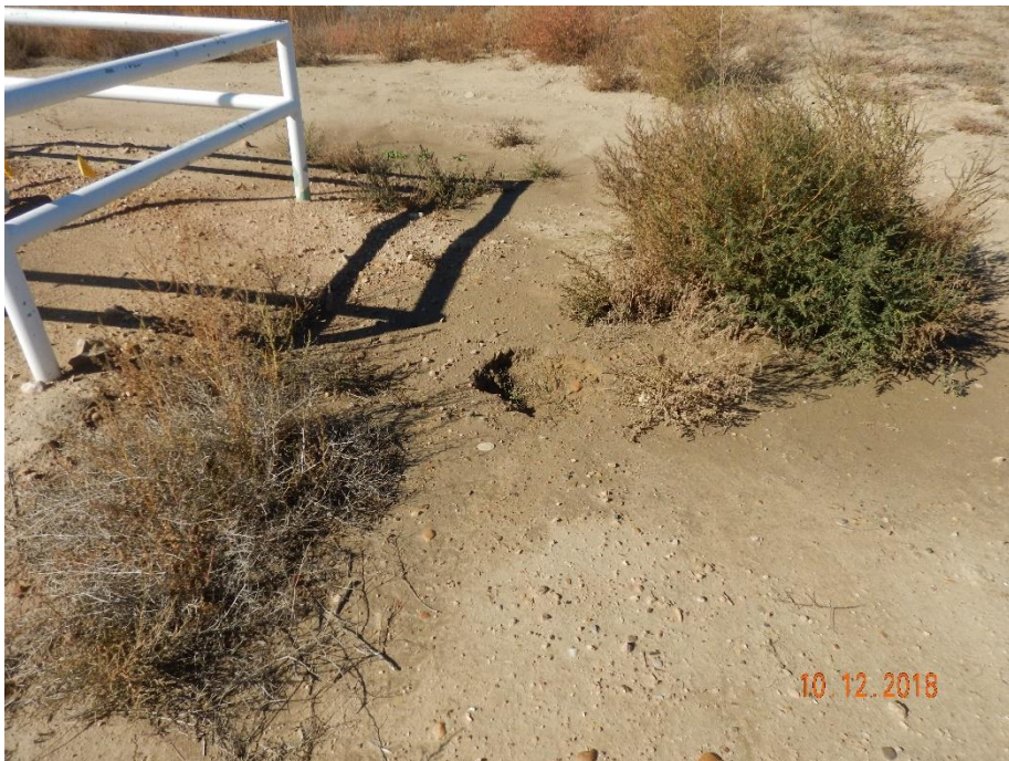
Photo 1: Photo taken from the battery location, facing west. Previous inspections documented subsidence concerns at the battery location and required operator to repair. Photo shows subsidence concerns remain.
