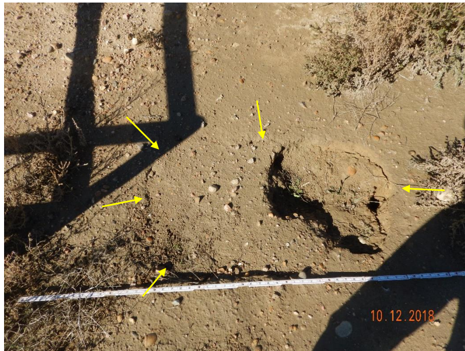
Photo 2: Photo taken from the battery location, facing west. Previous inspections documented subsidence concerns at the battery location and required operator to repair. Photo shows subsidence concerns remain and appear to be expanding. 6 foot measuring stick for reference.
