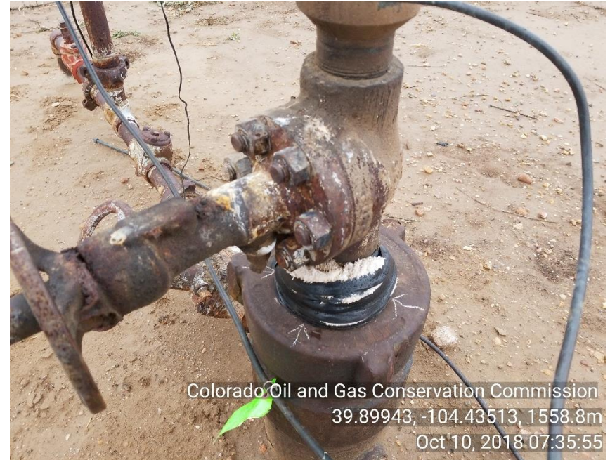
Photo 2 rags and electric tape around Plunger lift and WH
