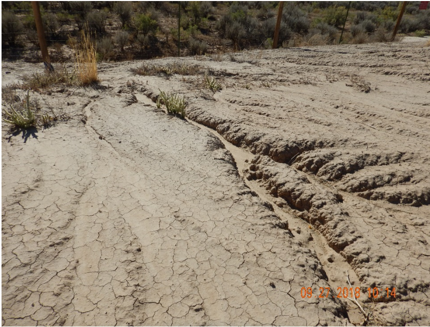
Photo #27 – Erosion rills along east berm of pit suggest apparent subsurface soil piping within berm.
