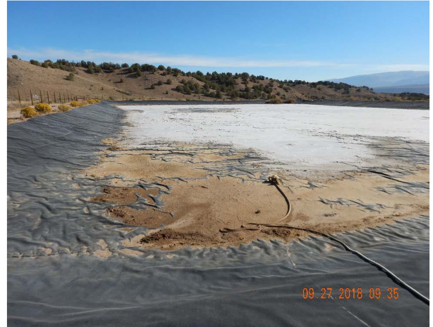
Photo #14 – Pit liner was covered in salt deposits and stained sediment on inspection date. Composite samples of sediment inside of pit exceeded COGCC Table 910-1 for multiple constituents, including DRO (doc #2144696).
