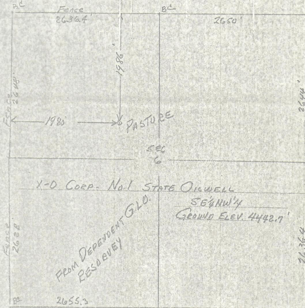
I hereby certify that the above plat is an accurate representation of a correct survey showing the location of X-O Corp.-No.1 State Oilwell in SE 1/4 NW 1/4 Sec. 6 T2N R54W 6PM. The elevation of the ground at the stake is 4442.7 feet above sea level from U.S.C.&G. Benchmark.
